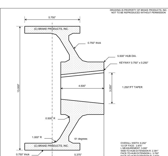
WEB-TO-HUB EXTENSION R: 2.391" FACE-TO-HUB EXTENSION L: 3.750" FACE-TO-HUB EXTENSION R: 2.500" APPROXIMATE WEIGHT (LBS.): 55 SMALL BORE DIAMETER: 2.781"
